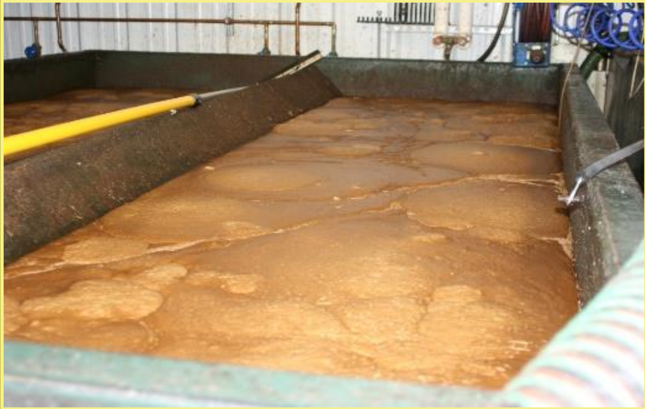
A vat of used cooking oil being processed into biodiesel at the Bently Biofuels plant in Minden. Photo by Kelsey McCutcheon.
